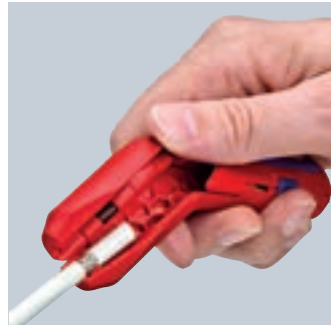
Stripping of a coax cable
