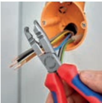
Cutting when shortening single conductors
